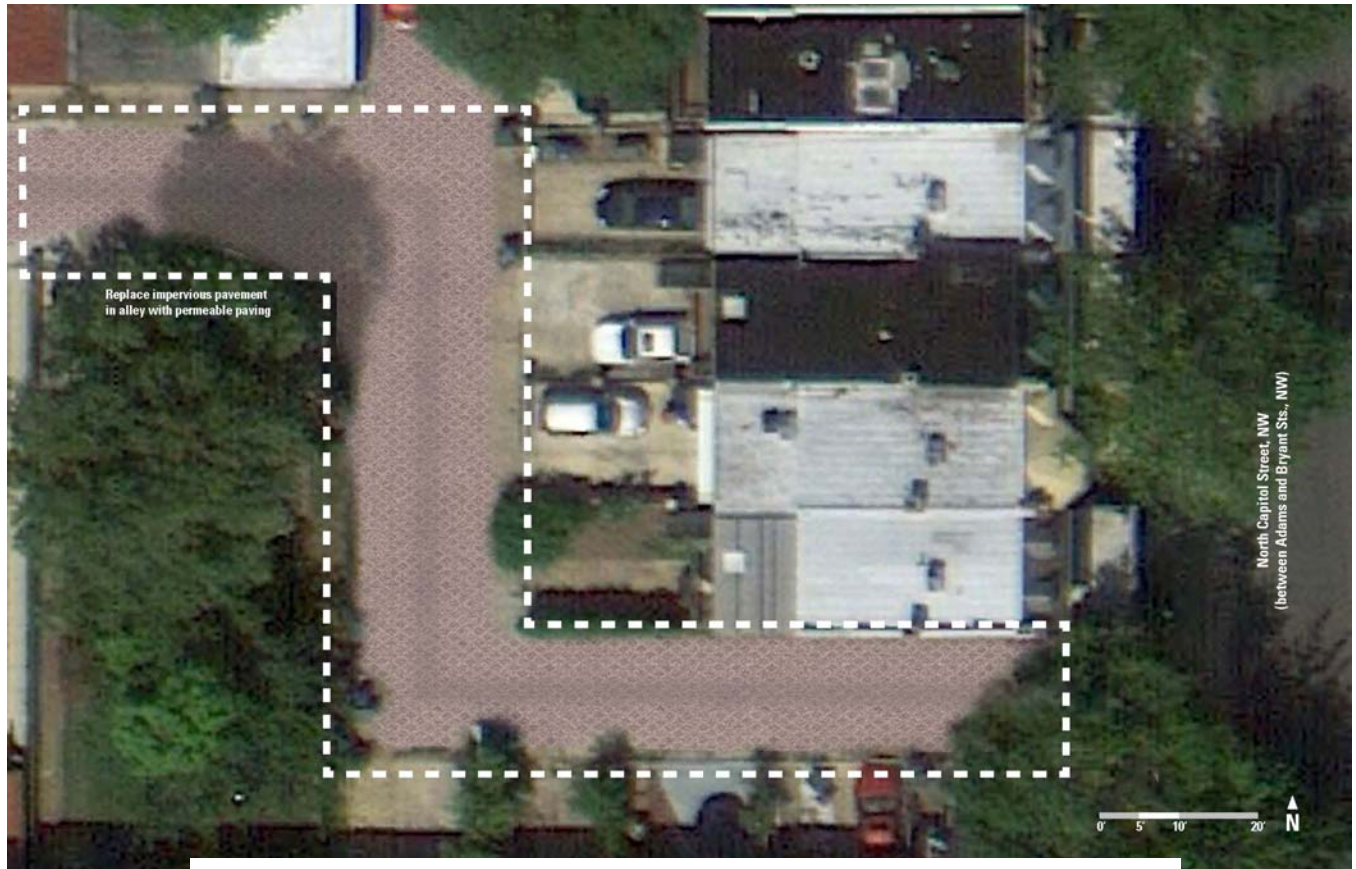
Figure 1: Proposed Green Street (Permeable Pavement in Alley) between Adams Street and Bryant Street NW, near North Capitol Street NW
