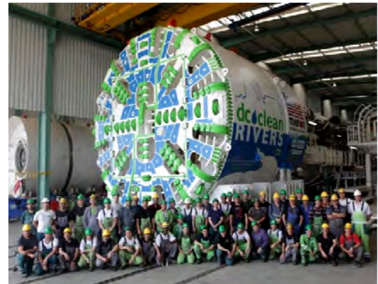
DCCR’s Tunnel Boring Machine (26-ft in Diameter).
