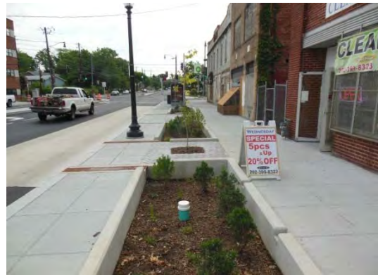
Bioretention practices include rain gardens, bio-swales, vegetated filter strips, and tree box filters
